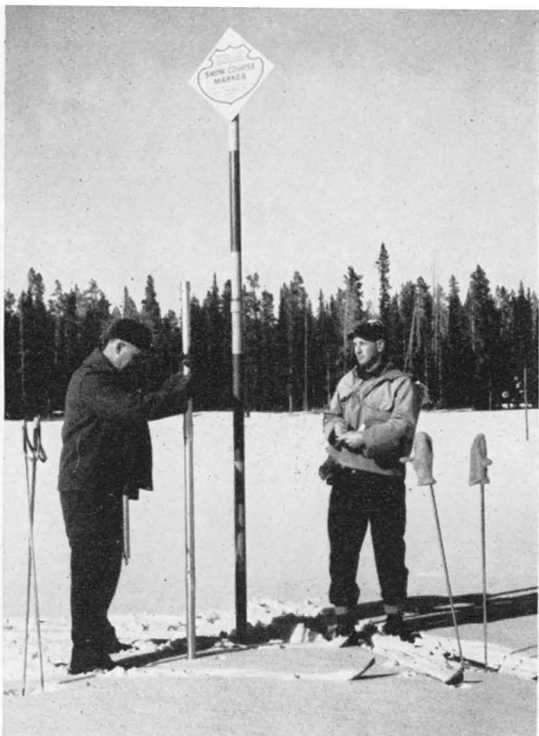
Out on the course a snow sample is taken by thrusting the Federal sampler—a 1 3/4-inch hollow, aluminum-alloy tube—down through many feet of snow to the ground beneath.
