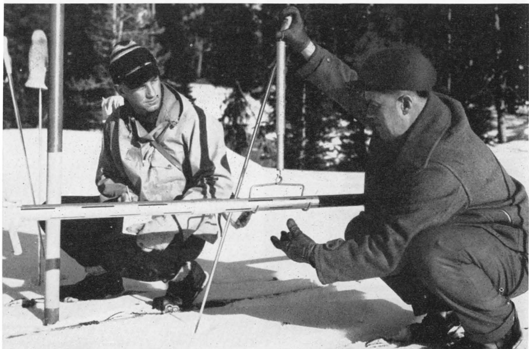
The sample is immediately weighed on special hand scales with markings that show the inches
