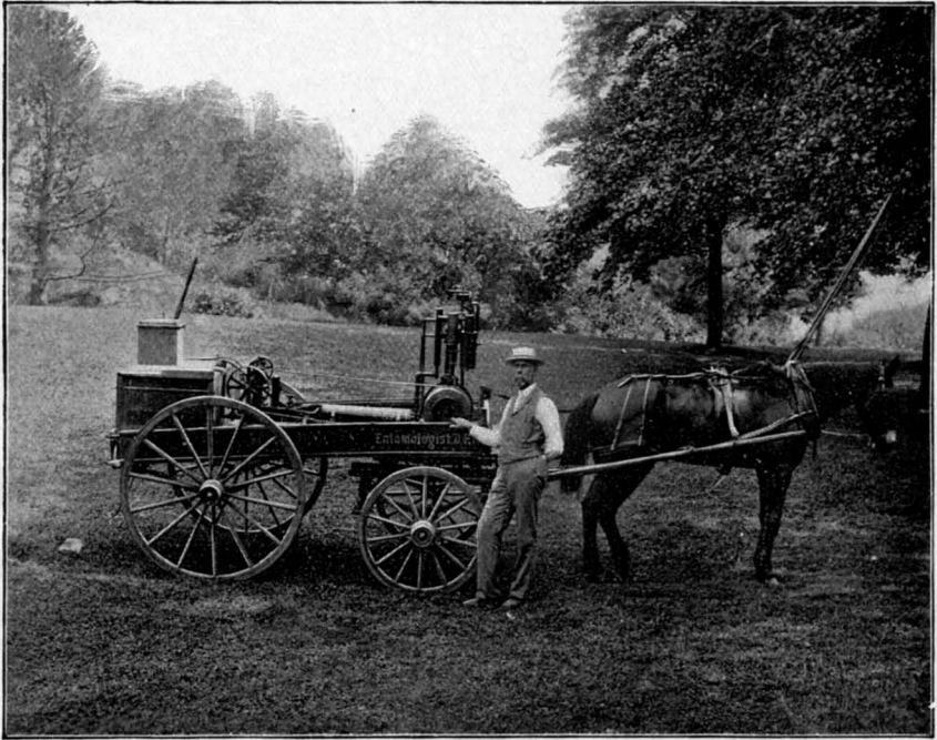
FIG. 1.—STEAM SPRAYING APPARATUS USED BY THE DEPARTMENT OF PUBLIC PARKS OF NEW YORK CITY.
