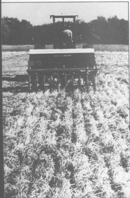
Lo-Till, an educational/research program, has become synonymous with minimum tillage in Oklahoma. Here, a wheat drill works its way through last season's stubble.
