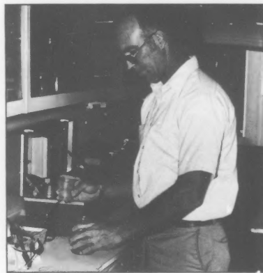
A mobile laboratory—converted from a camping vehicle—tests irrigation water from wells for total soluble salts, and other factors that can harm crops. Extension specialists from the University of Arkansas drive the lab, supervise testing of one hundred samples a day, and make recommendations to growers.
