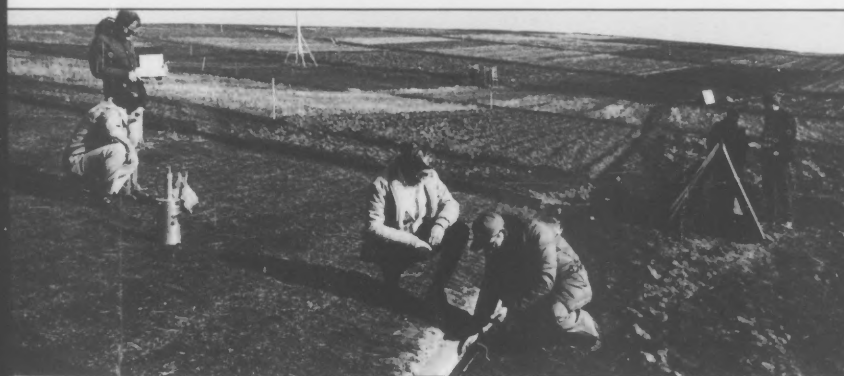
John Hammell (left), soil physicist, University of Idaho, and Rod Tittmore, scientific aide, measure soil moisture with a neutron probe. Robert McDole, Extension soil specialist, (Idaho), and Harry Riehle (center), SCS area agronomist, examine sediment. Edwin Dowding (right), engineer, (Idaho), explains the operation of a runoff collection device to Stephen Reinertsen, Extension associate, conservation tillage, (Idaho).
