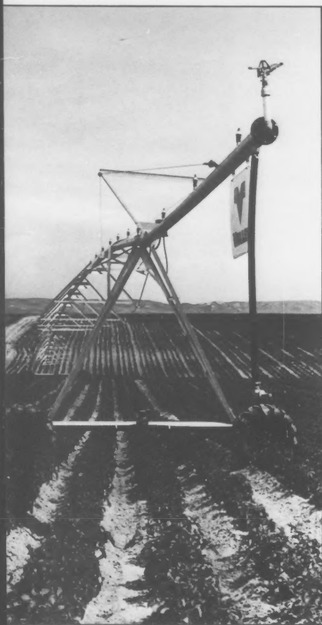
Left: A center pivot irrigation system in a Montana potato field; proper irrigation scheduling of such systems has a significant effect on water use and crop production. Below: A field scout records the depth of water in an evaporation pan in an irrigated barley field collecting important information about rainfall amounts between irrigations.
