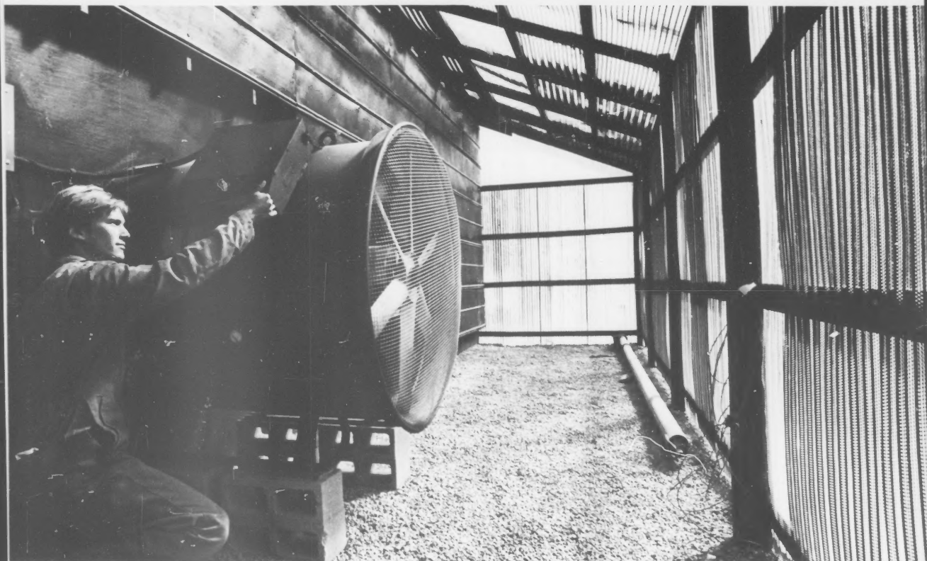
Mike Drewry, of Wakefield, Virginia, adjusts the fan in this unit designed for drying peanuts. Using available solar energy, preheated air enters the fan.
