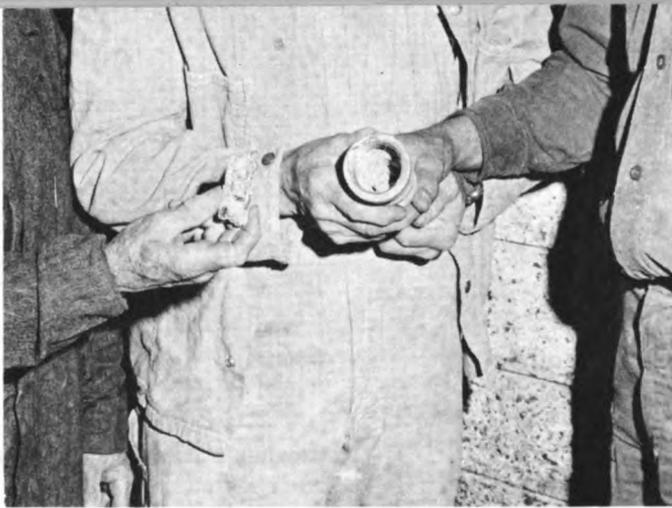
*Even in the best of barns, things happen to vacuum lines. A milk surge by high-producing cows plugged this line and produced the chunk on display.*
