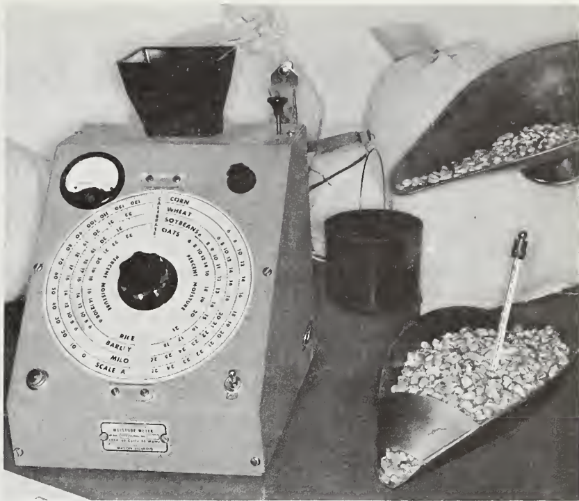
This special meter measures the moisture content of grain. It is used by SRS in the objective yield surveys. Corn, wheat, soybeans, and cotton are in the national program.
