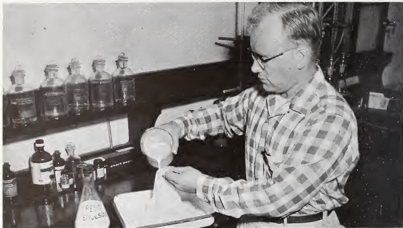
A chemist at the Southern Utilization Laboratory demonstrates soaking cotton cloth with an experimental wash-wear resin. He is wearing a wash-wear shirt that was washed and dried more than 20 times without ironing.
