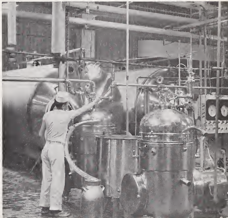
Shown here are twin separators in a new skim milk drying plant built as a result of merger of two Iowa firms.
