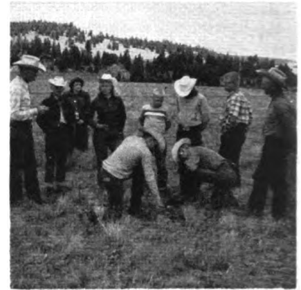
Karl G. Parker, extension range management specialist, tells 4-H Club members how to use an infiltration ring to measure the rate at which water sinks into range soil under various plant cover conditions.
