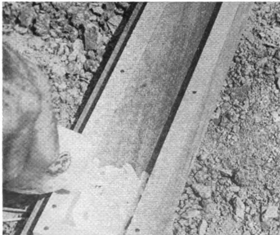
Apply adhesive to as much of the tray as the soil samples will occupy.
