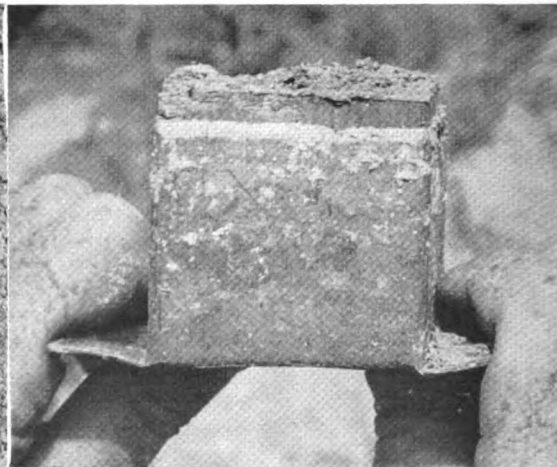
Remove the block of soil from the sampler by pushing out the stopper block.
