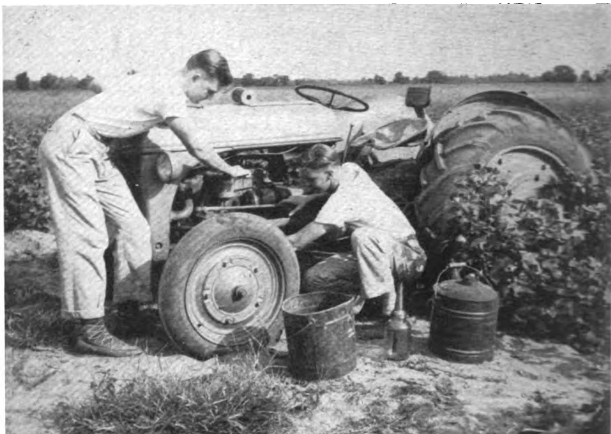
Joe Beck and Frank Stanley of Henry County, Mo. demonstrate how to change oil filters on a tractor.
