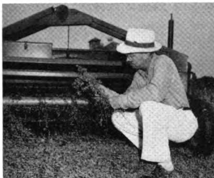
Higher yielding alfalfas, like Atlantic, can supply even more feed nutrients per acre when the mower-crusher, shown above, is used. Crushed by the heavy rolls, the alfalfa stems dry quicker and retain more of their feed value.
