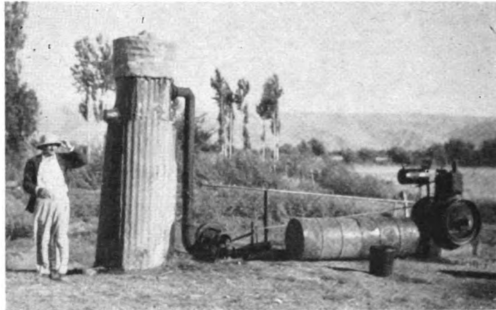
Power pumps, used to pump water to irrigate the land, are an important factor in increasing production in the Bekaa Valley. This pump supplied most of the water needed for drinking and cooking in the village of Marj.
