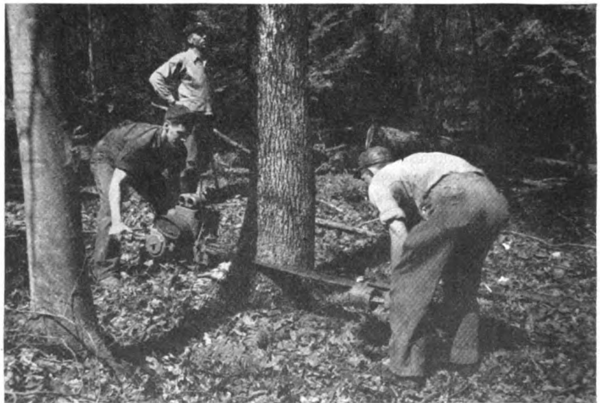
Power saws make it easier to cut low stumps—a good forestry practice which also provides closer utilization.
