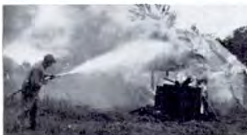
This demonstration of fighting fire with the orchard spray rig is typical of those given in Michigan.
