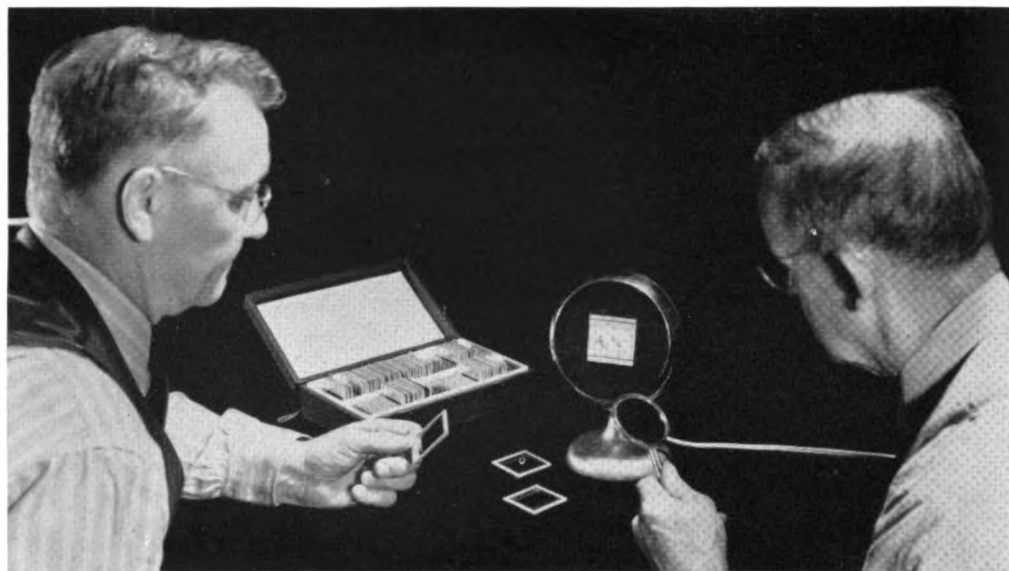
Single-slide illuminator made by County Agent R. M. Gridley, Beaver County, from a discarded automobile spotlight.
