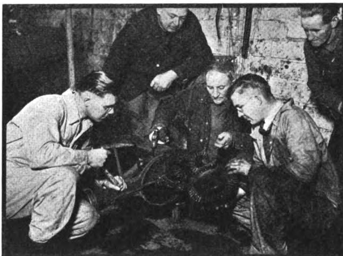
Byron T. Virtue, extension agricultural engineer in Iowa (lower right), shows local leaders, including the owner of the mowing machine, how to adjust the bevel gears so that they will mesh to the proper depth.
